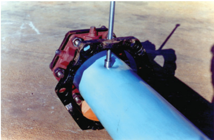
1.5 inch Penetration of Tup into 6.90 inch Diameter Pipe Wall, 0.38 inch Thick, 70° Ambient Temperature
